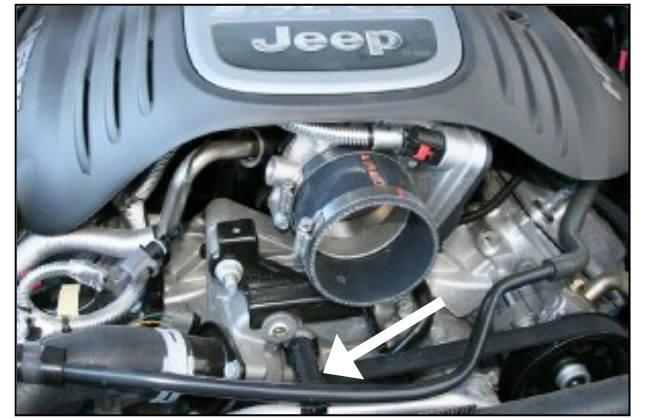
15. Install the coupler and two #60 hose clamps on the throttle body as shown. Do not tighten the clamps at this time. Secure the breather hose to the air conditioner line using the supplied zip tie.
