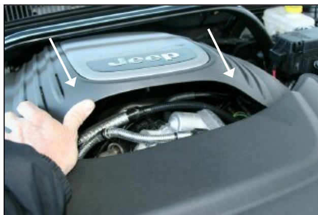
20. Realign the engine cover with the grommets on the engine, and push down firmly to reseat the cover.
