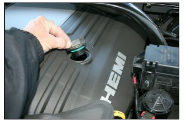
21. Reinstall the oil fill plug. 22. Recheck your work, make sure there is no foreign material in the intake, double check all hose clamps, screws and nuts for tightness. 23. Reconnect the negative battery cable.
