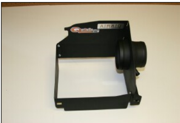
11. Assemble the two pieces of the Quick Fit panels as shown, using the four 6-32 screws, washers, and nuts, that are provided in the kit. Apply the Airaid Foil Decal onto the Panel as shown.
