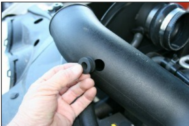
16. Install the supplied grommet into the hole in the back of the tube.
